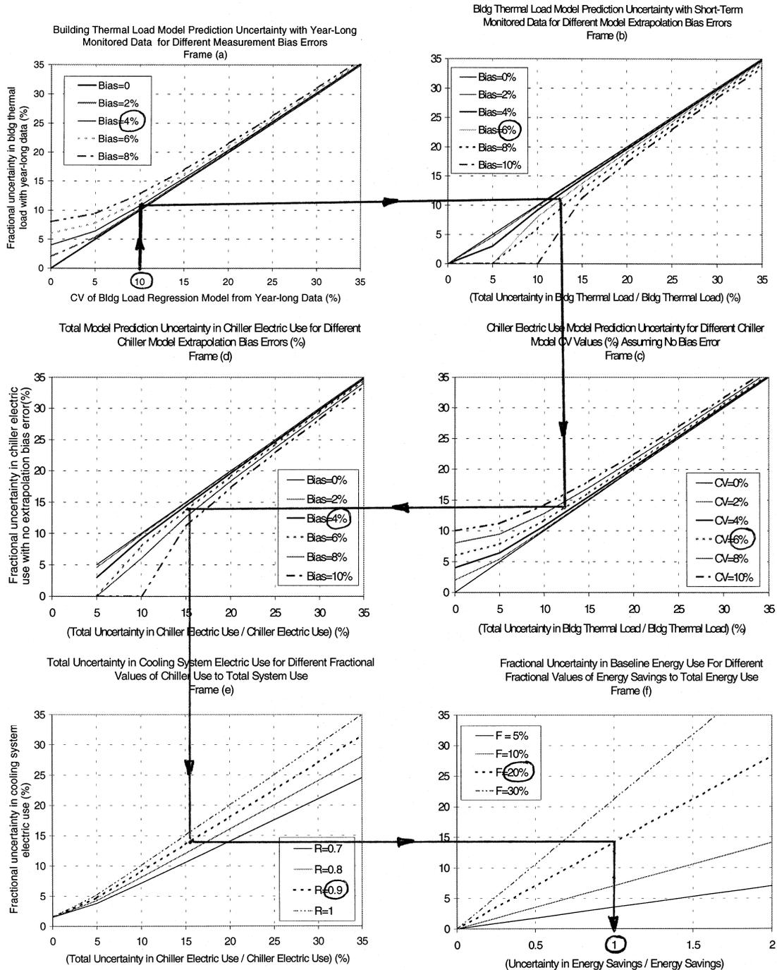
**Figure 4** Nomograph to determine the final uncertainty in energy or cost savings of a cooling system due to various individual measurement and regression model prediction uncertainties. An illustrative example as explained in the text is also shown.
