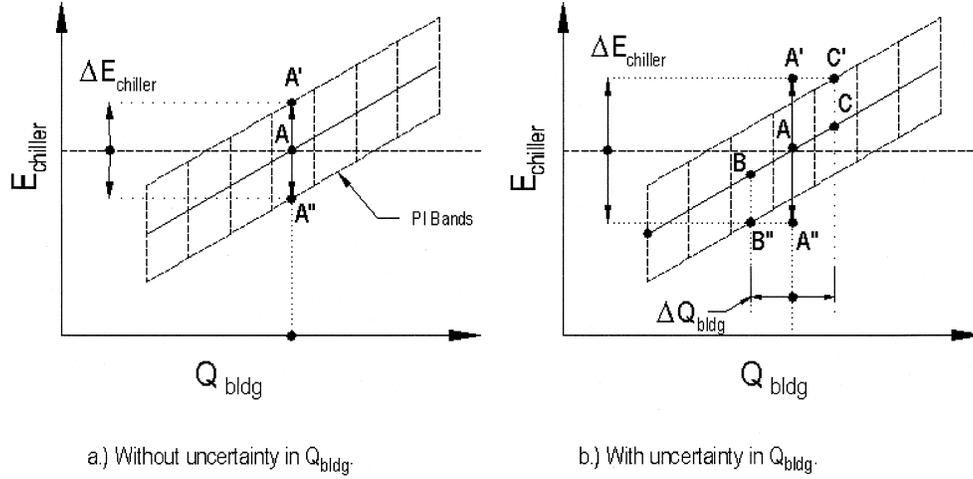
**Figure 3** Conceptual plot to illustrate how one could include the uncertainty in building secondary loads while determining uncertainty in chiller electric use assuming a simple linear relationship to exist between both variables.
