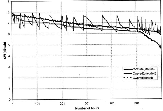
**Figure 2** Load duration curves of measured chilled-water energy use and that predicted by using the SMLP method for all hours during summer using the ASHRAE Predictor Shootout II data.
