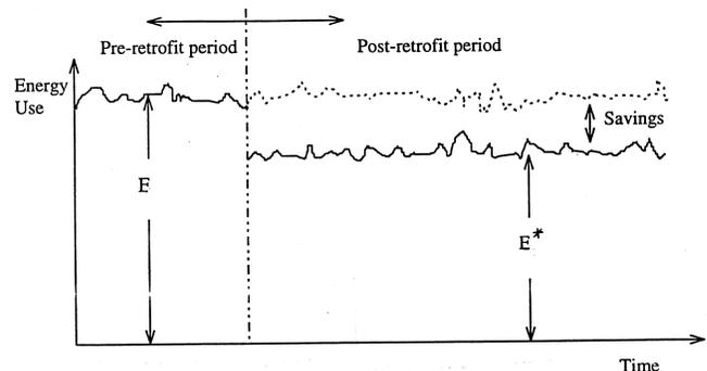
**Figure 1** Conceptual plot showing relationship between energy savings and energy use before and after the ECM.
