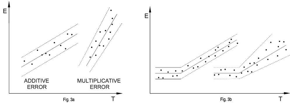
**Figure 3. Conceptual plots to illustrate additive and multiplicative errors in linear and change-point three parameter-cooling models**
