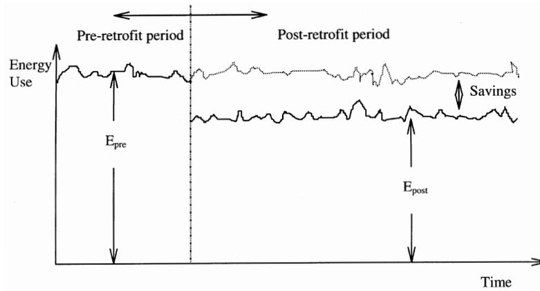
**Figure 4. Conceptual plot showing how energy savings are determined**
