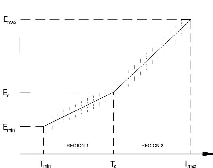
**Figure 2. Illustration of data points fitted by a change-point four-parameter cooling model (4P-C)**
