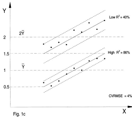
**Figure 1. Conceptual plots to illustrate how different configurations of linear data affect model  $R^2$  and CVRMSE**
