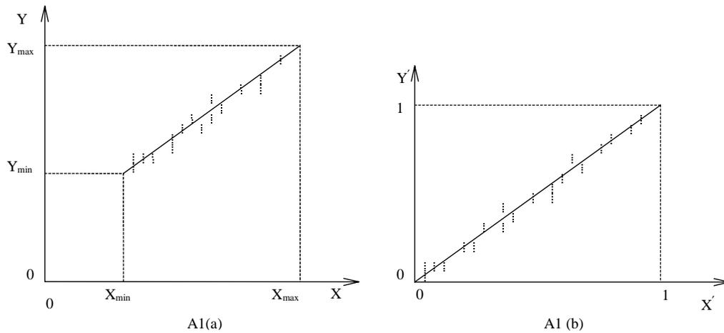
**Figure 6. Transformation of linear model to fit into square with origin (0,0) and (1,1) as other end point**
