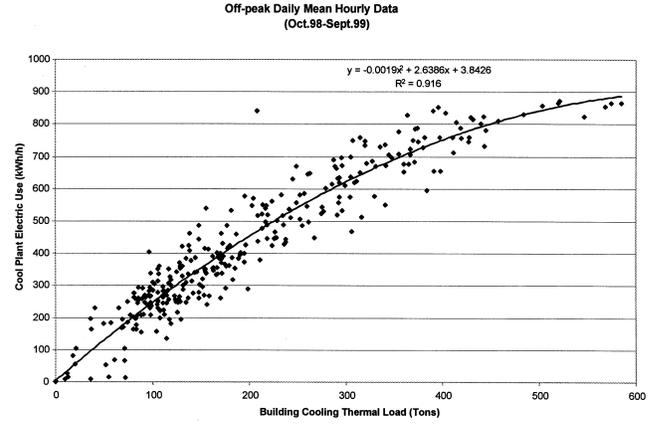
**Figure 4b** Scatter plot of daily mean hourly cooling plant electricity use vs. thermal cooling load during off-peak period for the whole year—Case Study #3.
