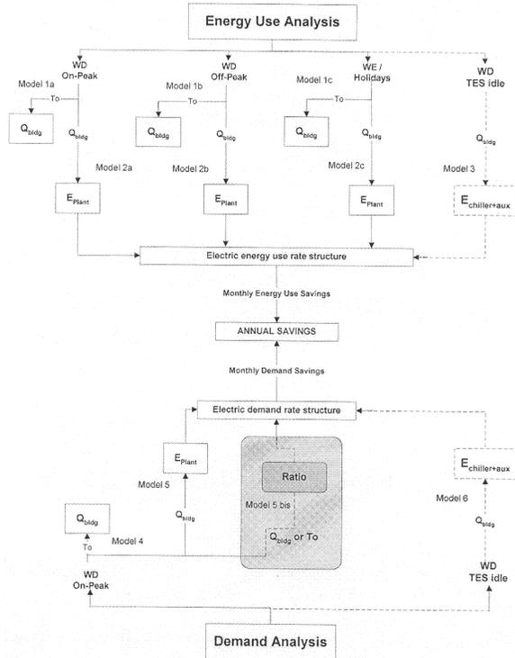
**Figure 1** Flow chart of the basic lumped model analysis approach to characterize actual cooling plant performance.
