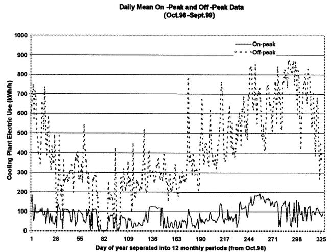
**Figure 2c** Time series plots of daily mean data from October 1998 to September 1999 separated into on-peak and off-peak periods: cooling plant electricity use (kWh/h)—Case Study #3.
