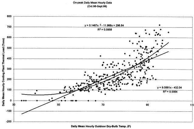
**Figure 3a** Scatter plot of daily mean hourly thermal cooling load vs. outdoor temperature during on-peak period for the whole year—Case Study #3.
