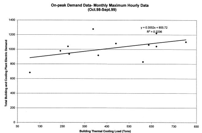
**Figure 6** Scatter plot of monthly peak facility (building plus cooling plant) electric demand vs. building thermal cooling load during on-peak period—Case Study #3.
