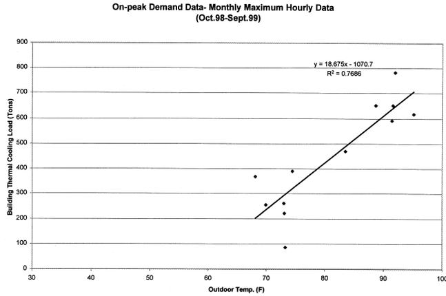
**Figure 5a** Scatter plot of monthly peak hourly building cooling thermal load vs. outdoor temperature during on-peak period—Case Study #3.
