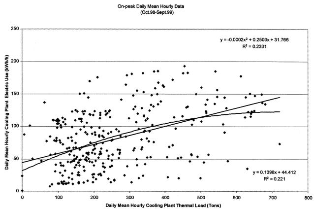
**Figure 3b** Scatter plot of daily mean hourly cooling plant electricity use vs. thermal cooling load during on-peak period for the whole year—Case Study #3.
