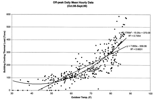
**Figure 4a** Scatter plot of daily mean hourly thermal cooling load vs. outdoor air temperature during off-peak period for the whole year—Case Study #3.
