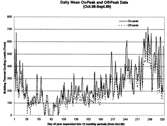
**Figure 2b** Time series plots of daily mean data from October 1998 to September 1999 separated into on-peak and off-peak periods: building thermal cooling load (Tons)—Case Study #3.
