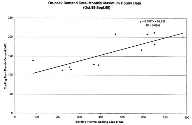
**Figure 5b** Scatter plot of monthly peak hourly cooling plant electricity use vs. building cooling thermal load during on-peak periods—Case Study #3.
