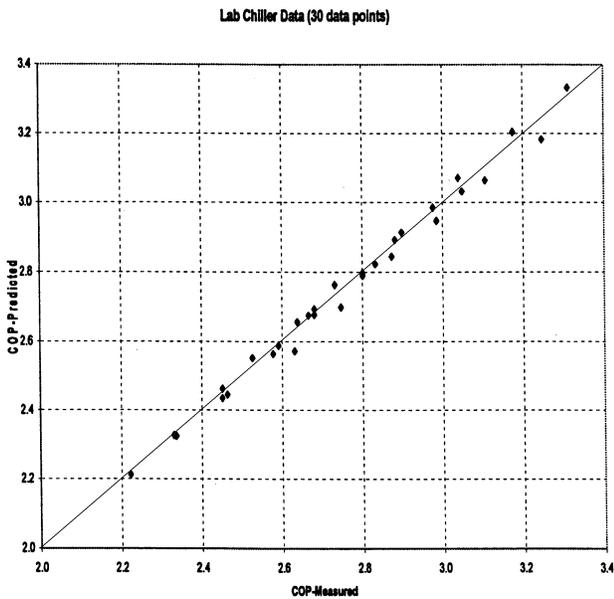
**Figure 4** Prediction accuracy of the GN chiller model identified from four data points following the selection procedure proposed in this study.
