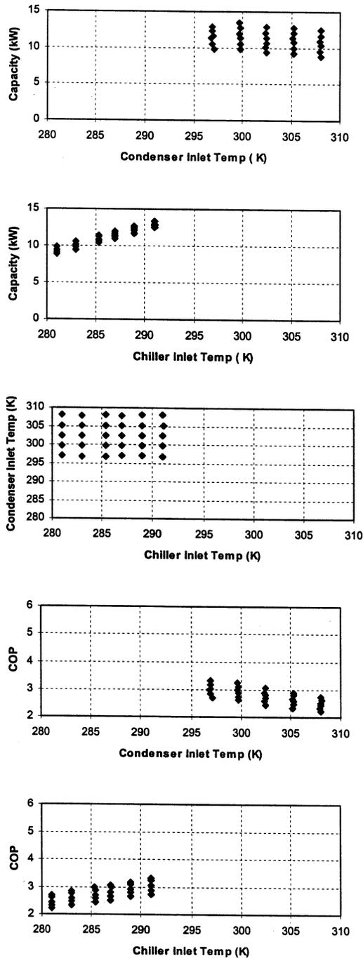
Figure 1 Laboratory chiller data (30 data points).
