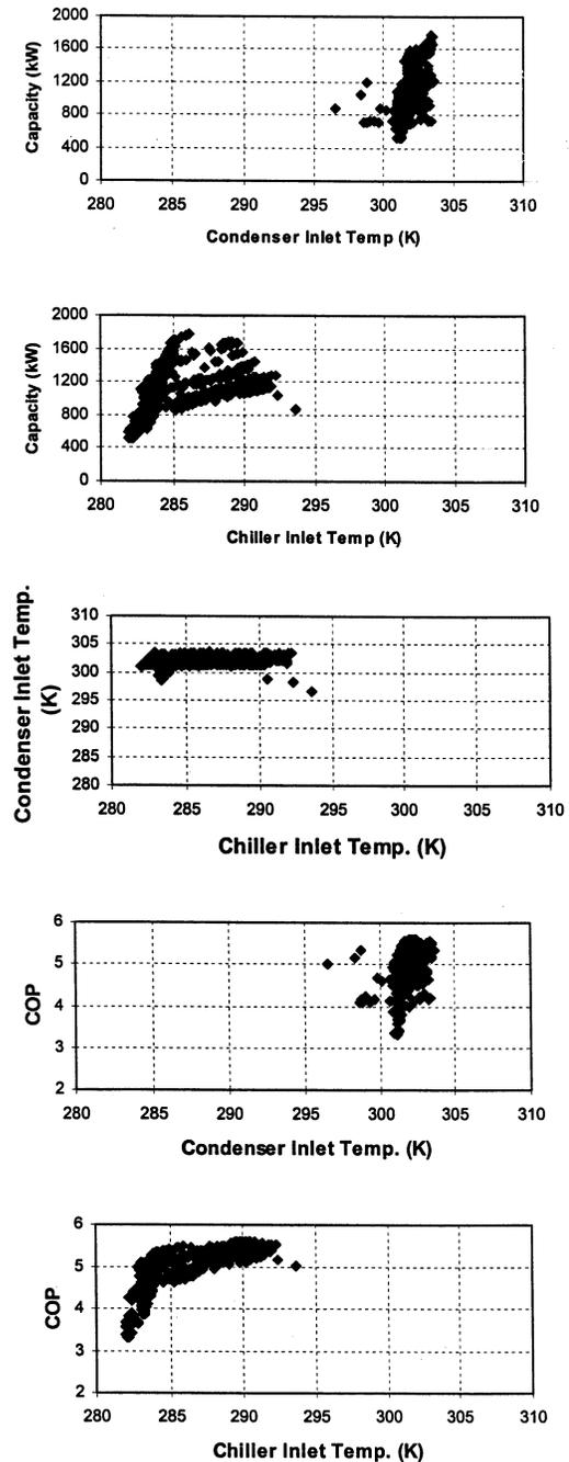
Figure 2 Field-operated chiller data at Toronto (810 data points).
