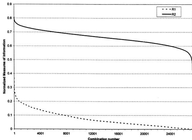
**Figure 3** Values of the ratios  $R_1$  and  $R_2$  defined by Equation 11, sorted by descending order, for the lab chiller data. The x-axis represents the number of combinations of 30 data points taken 4 at a time.
