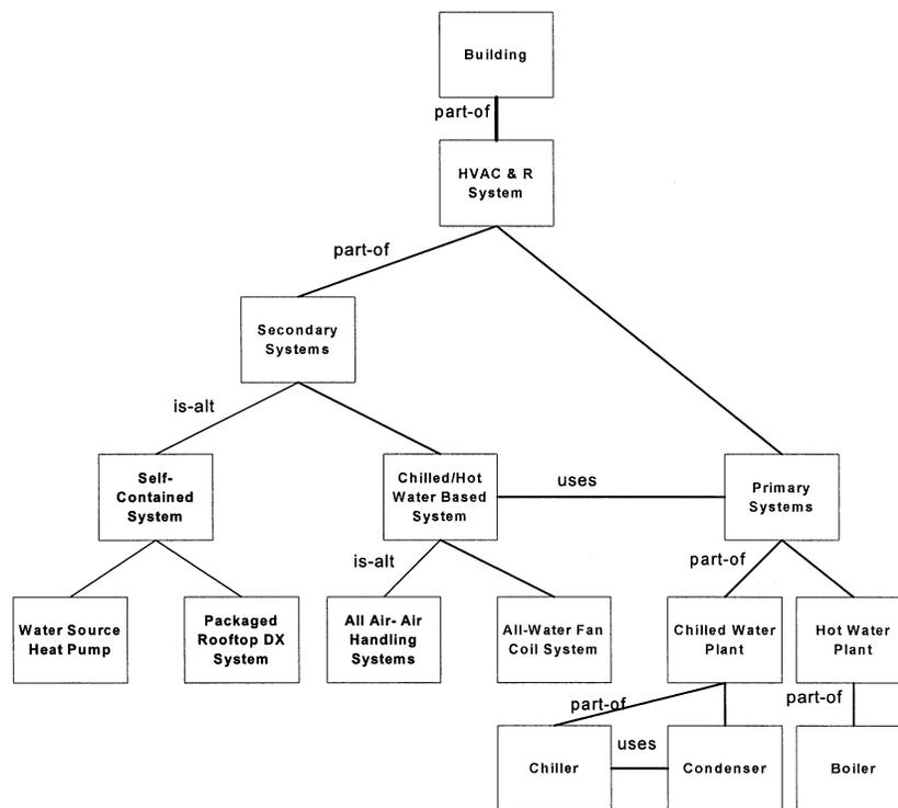
**Figure 3** Example of semantic network knowledge representation in HVAC&R design alternative involving a fan coil system.
