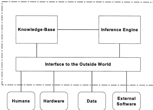
**Figure 4** Typical structure of a knowledge-based system.
