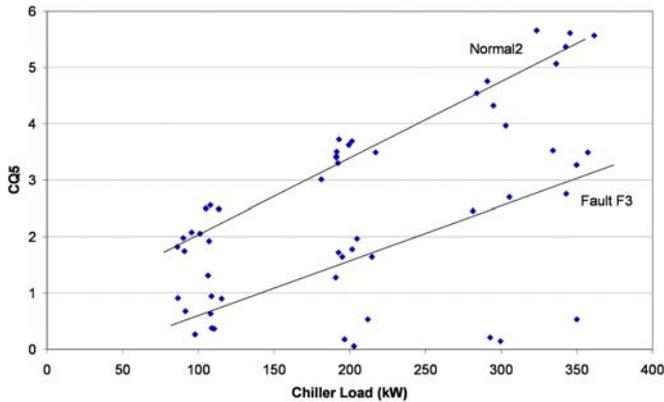
Figure 2. Scatter plots with trend lines illustrating how refrigerant loss (fault F3) at severity level SL4 impacts the variable CQ5 with respect to the fault-free behavior.
