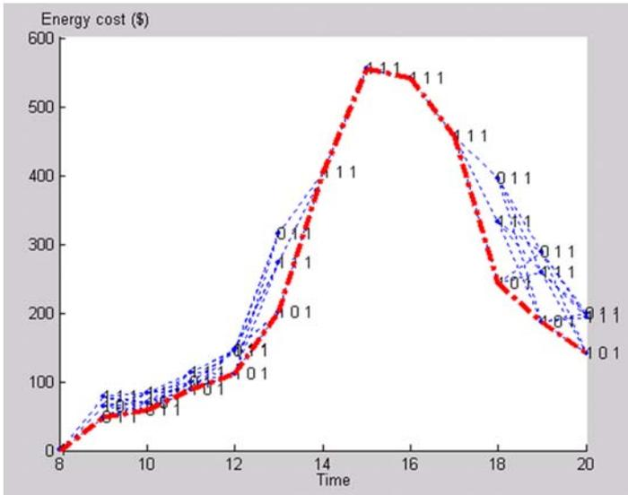
Figure 5. Chiller scheduling under diurnal condition RTP-1. The bolded dash-dot line represents the least-cost path (or chiller operating strategy) and the dashed lines represent the various feasible scheduling strategies over the planning horizon. The labeled numbers beside the lines denote the chiller feasible operating modes (groups).
