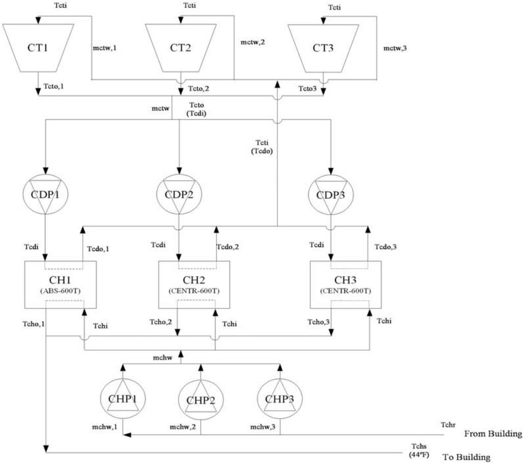
**Figure 1. Schematic of the hybrid cooling plant assumed for the case study.**
