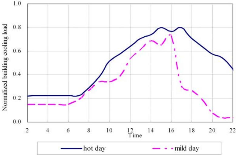
**Figure 2. Normalized building cooling load profiles for a typical hot day in June and a typical mild day in September in Philadelphia.**
