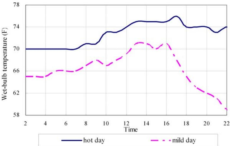
**Figure 3. Wet-bulb temperature profiles for a typical hot day in June and a typical mild day in September in Philadelphia.**
