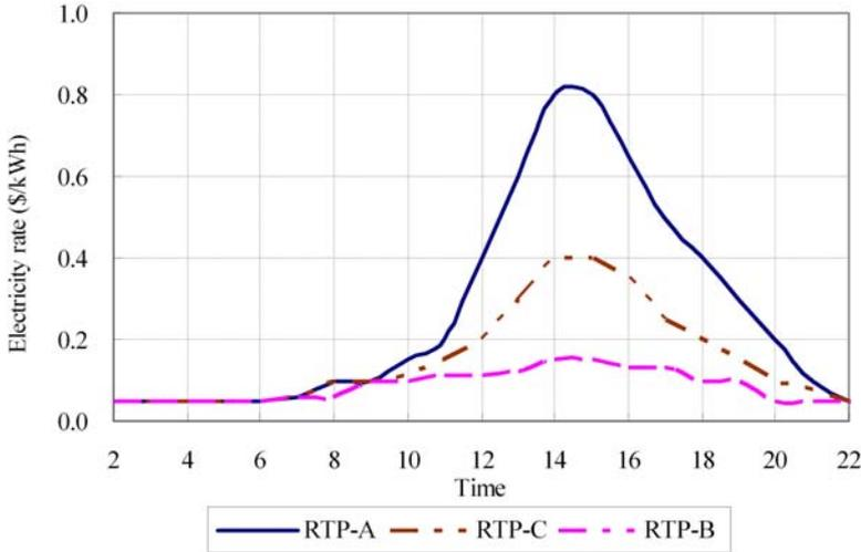
**Figure 4. Typical daily RTP profiles of electricity rates (adapted from Henze and Krarti [1999]).**
