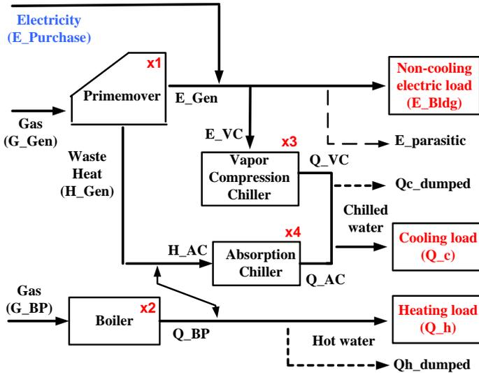
**Figure 1. Generic schematic of the BCHP system depicting sub-system interactions and nomenclature used. The terms x1, x2, x3 and x4 represent the loading fractions of the primemover(s), boiler(s), vapor compression chiller(s) and the absorption chiller respectively.**
