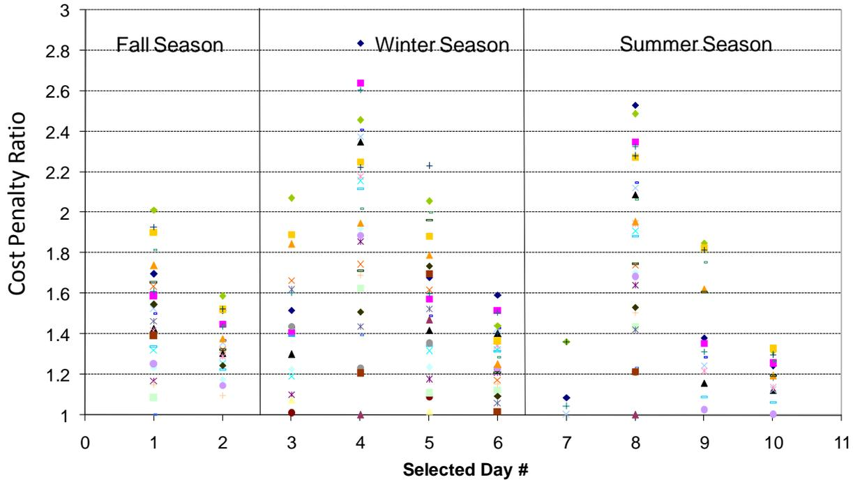
**Figure 5.** The spread in excess operating costs characterized by CPR during the 10 selected days over the 15 hour diurnal time horizon. Though there are 36 possible system combinations, only the results of the feasible system combinations are shown.
